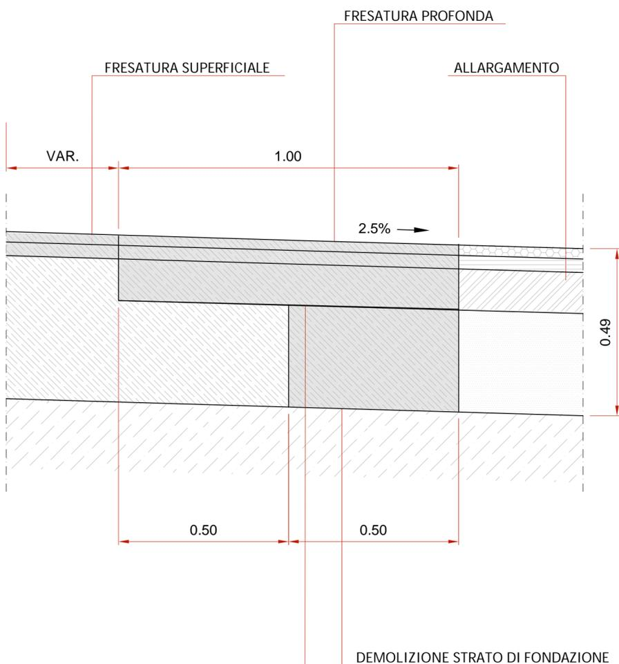
STRUTTURA DI RINFORZO COSTITUITA DA GRIGLIA COMPOSITA BITUMATA IN FIBRE DI POLIESTERE AD ELEVATO MODULO ACCOPPIATA AD UN GEOTESSILE ULTRA LEGGERO IN POLIPROPILENE
