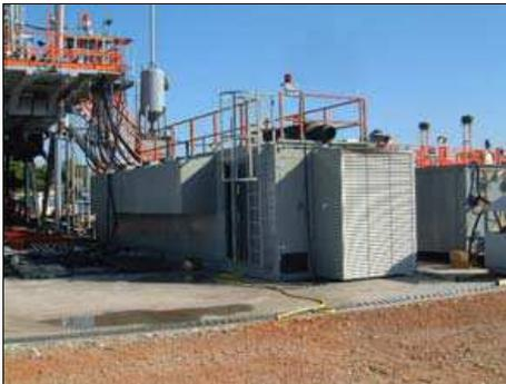
*Figura 7 – Una power unit DRILLMEC 1000*
