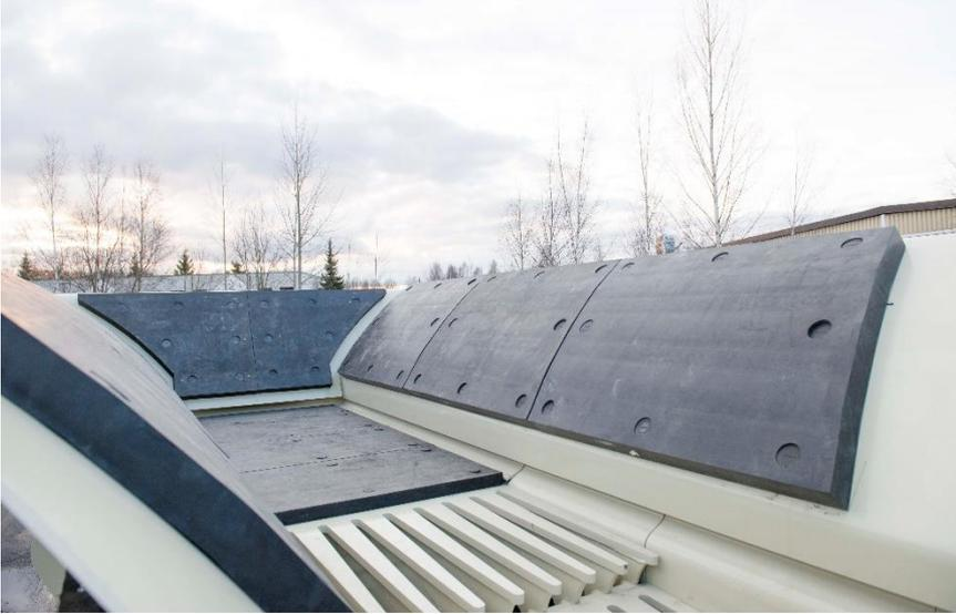
Rubber lining for hopper sides and feeder bottom - Reducing noise and improving material flow in sticky applications
